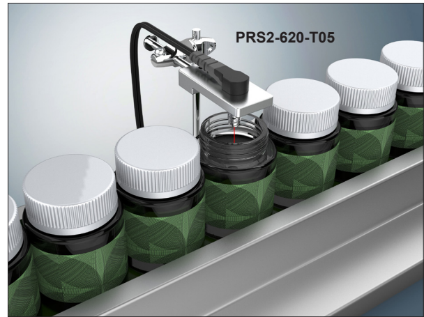
檢測有無蓋子 Detecting presence of cap.
