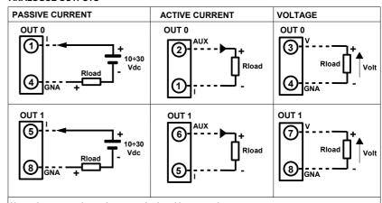
Note: the output channels are not isolated between them. Terminals AUX of channels connected between them. Terminals GNA of channels connected between them
