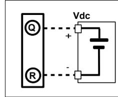
(\*) Note: for UL installation the device must be powered using a power supply unit classified NEC class 2 or SELV
