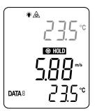
The meter works in air velocity measuring mode (please refer to chapter 6-1). Place the sensor in the air stream. It will show the air velocity value on the primary reading and show the air temperature value on the tertiary reading. During measuring, press the " button once to hold the air velocity value and the" "HOLD" symbol will appear on the LCD.
