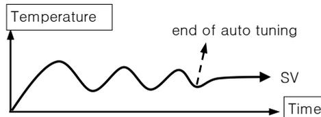
\*Auto tuning will be finished, after repeating 3 times of OFF over 2°C of SV value after ON below 2°C of SV value.
