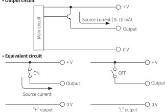
Connection example of PNP open collector output type and external
