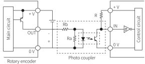
• Use low resistance for Ra and Rb values within the range that does not exceed the rated load current of the rotary encoder.
