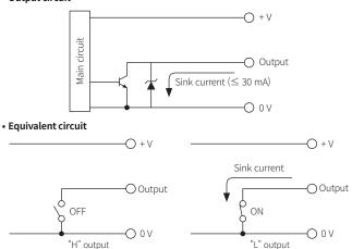
Connection example of NPN open collector output type collector and counter
