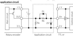
CMOS IC circuit • Use low resistance for Ra and Rb values within the range that does not exceed the rated load current of the rotary encoder.
