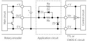
• If input voltage of control circuit is lower than applied voltage of encoder
