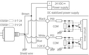
PLC DC input circuit
