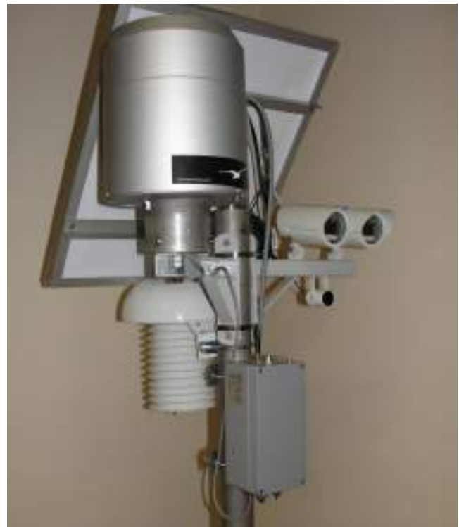
GSM-2 box* (below) with rain catcher at a testing site in the Novgorod Oblast
