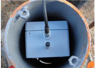
GSM-2 box\* remote transmitter with data logger
