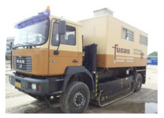
Special trucks used for cone penetration testing
