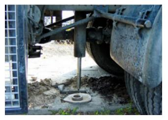
The cone is pressed into the ground
