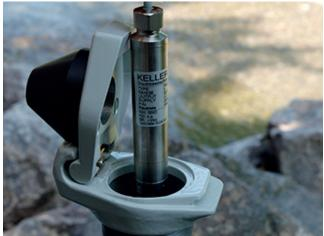
Sensor in a DCX-22 AA data logger
