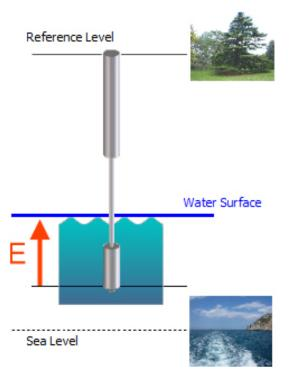
Water column calculation using a membrane
