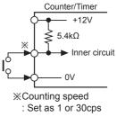
%CP1, CP2 (INHIBIT), RESET input part
