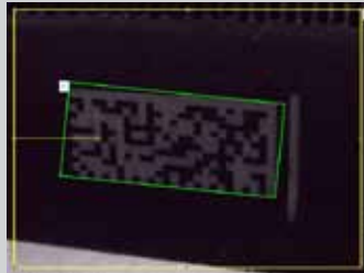
Low-contrast code Code is made legible through high tolerance – also towards weakly contrasting codes.
