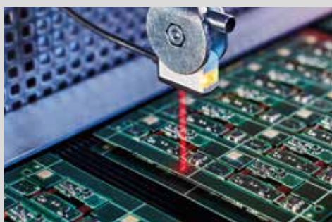
Detecting double layer of printed circuit boards, or presence and height control of components
