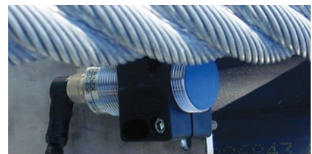
Distance monitoring for position control
