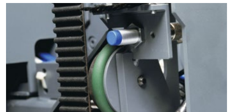
Drive-belt tension monitoring
