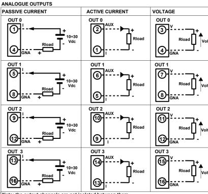
Note: the output channels are not isolated between them. Terminals AUX of channels connected between them.
