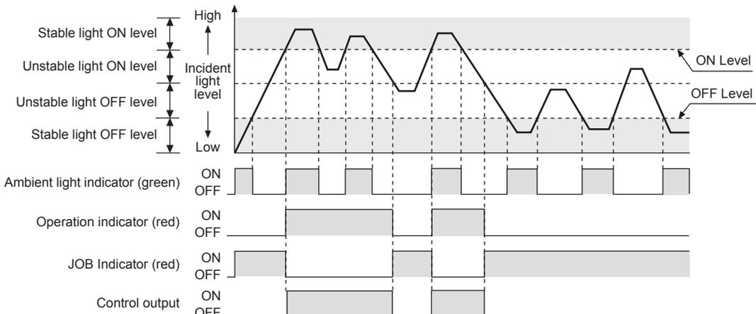
※The waveforms of operation indicator, job indicator, and control output are the state of operation for Light ON, but in case of Dark ON, it is opposite operation against Light ON mode.
