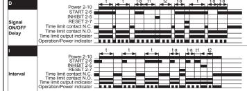
XIf power is cut or the RESET terminal is short-circuited, the timer will be reset XIf the INHIBIT terminal is short-circuited during a time limit operation, the time will stop. XIn case of F, F1 output operation mode, setting time should be over 100ms.
