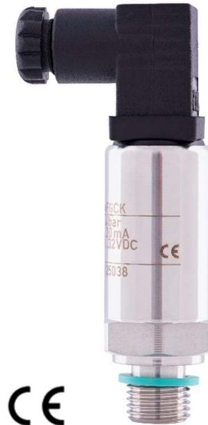
The HOM Series offers the robust design with stainless steel housing of the HOT Series but uses a silicon based sensitive measuring cell for low pressure applications from 10 mbar to 500mbar. With additional EMI / RFI protection, low static and thermal errors and high resistance to shock and vibration as standard, the HOM Series assures trouble free operation at temperatures up to 85°C.
