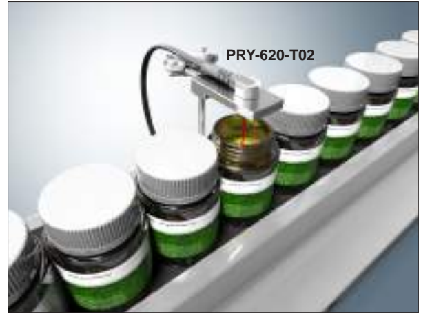
檢測有無蓋子 Detecting presence of cap.
