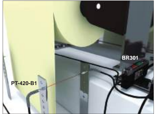
檢測紙張邊緣 Detecting edge of paper.
