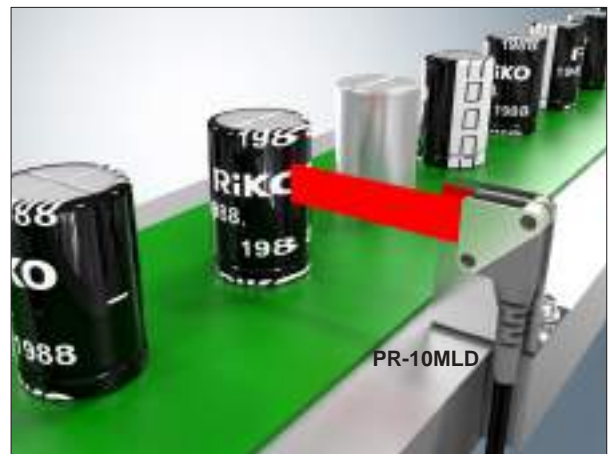
檢測電容是否缺損 Detecting capacitor deflection.
