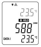
The meter works in air flow measuring mode (please refer to chapter 6-2). Place the sensor in the air stream. It will show the air flow value in the primary reading and show the air temperature value in the tertiary reading. During measuring, press the "" button once to hold the air flow value and the " HOLD "symbol will appear on the LCD. Press the button again to return to normal operation.
