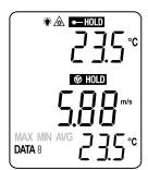
In measuring mode, press the "button to toggle the "MAX/MIN/AVG" mode and measure a target, it will show the MAX/MIN/AVG air velocity (flow) value on the primary reading and show the MAX/MIN/AVG temperature value on the secondary reading.
