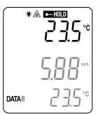
The meter works in temperature measuring mode. To measure, press the "button and point the meter at the target. It will show the temperature value on the secondary and the symbol will appear on the LCD after release the "button."
