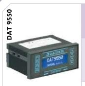
The device DAT 9550 is a graphic display designed for panel mounting and communicating with Modbus RTU protocol on RS-485 and RS-232 serial Slave port. Moreover on the device there is a RS-485 Master port by means of which it is possible to communicate with the eventual Modbus Slave devices connected. It can be used as Slave peripheral for the visualization of the data coming from the Intelligent Units of the DAT9000 series or from a PC, PLC or panel operator.
