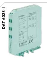
The devices of the DAT6000 series are an evolution in the techniques of connection of analog signals to PLC.
