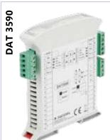
The device DAT 3590 is an isolated repeater between asynchronous serials lines RS485 or RS422 that guarantees a full isolation between power supply and serial line removing eventual ground-loop effects, allowing the use of the device even in the heavy environmental conditions. It is designed to operate either on serial interface RS-422 full-duplex 4 wires or RS485 half-duplex 2 wires, with a baud-rate transmission up to 115.2 Kbps.
