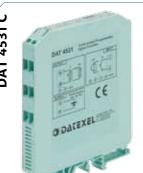
The isolated converter DAT 4531 C is able to measure and linearise the standard PTC and NTC sensors and potentiometers. In function of programming, the measured values are converted in a current or voltage signal. The device guarantees high accuracy and performances stability both versus time and temperature.
